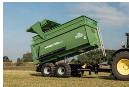
TA 20053/2 PT+ with conical trough, made of 4 mm thick sheet steel
