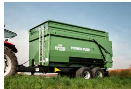
TA 14045/2 PT+ with 2 tipping cylinders for optimum tipping stability
