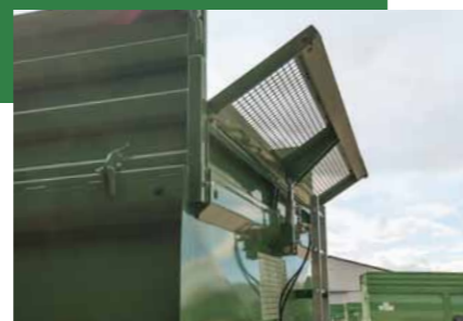
Front wall hydraulically foldable
