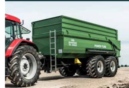
TA 22053/2 XPT+ continuous 6 mm sheet steel, height 1000 mm
