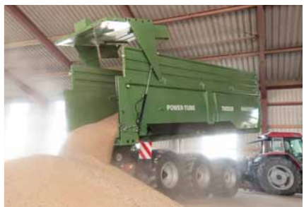
TR 34080/2 PT+ 34 t total weight, with hydraulic-mechanical or electric forced steering on request
