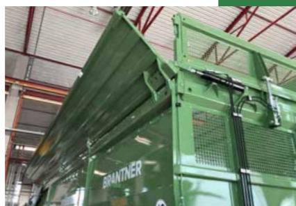
hydraulically foldable attachment wall optionally on the left or right side
