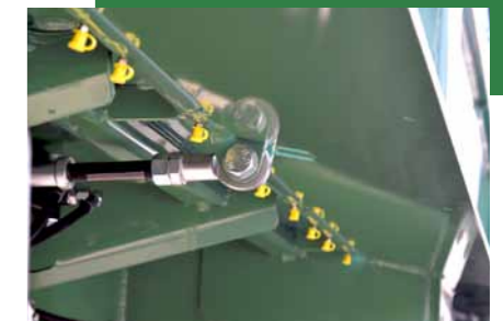
Innovation by Brantner Hydraulically controlled pendulum function for opening and closing
