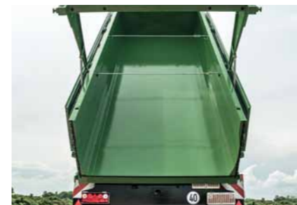
conical through for easier slipping of the load
