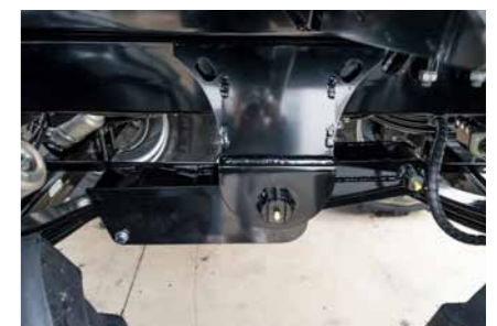
offset tandem unit Suspension on steering axle adjusted, better stability and reduction of the roll tendency
