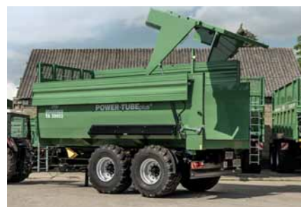
fold-down attachment walls Hydraulic rear wall can be opened when the top walls are folded down
