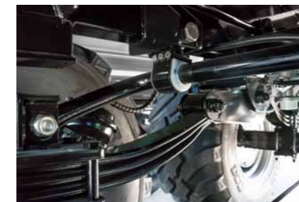
Spring stabiliser Highly recommended for steering axle (only possible with parabolic suspension)
