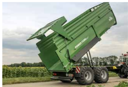
TA 24080/2 PT+ Body length 8000 mm, with air suspension and automatic tipping lowering as standard
