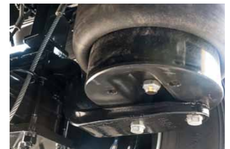
Air suspension with two-blade handlebars for optimum stability and off-road mobility
