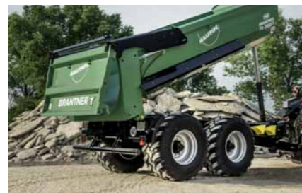
hydraulic pendulum flap Double-acting hydraulic rear wall opening with double function
