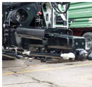
hydraulic-mechanical forced steering
