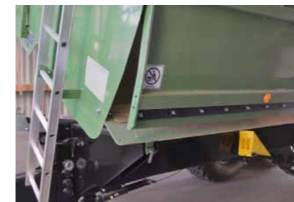
Slide for gentle unloading via laterally folding slide
