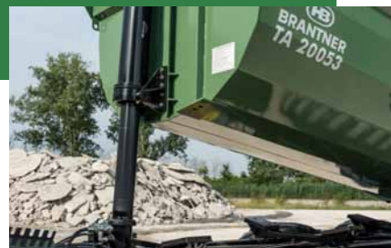
Front cylinder Hard-chrome plated for particularly high lifting force and tilt angle over 50 degrees
