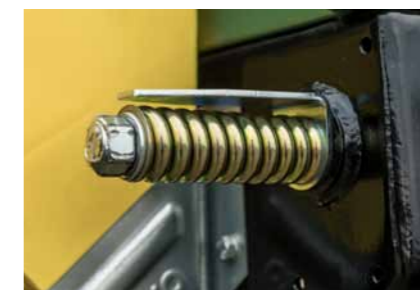
BRANTNER advantage automatic chain tensioner as standard
