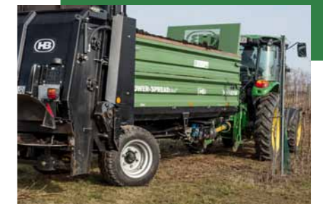
Innovation by Brantner optional hydraulic steering axle
