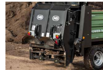
Universal spreading unit the CL2-2 compost spreader with two horizontal milling rollers and spreading discs
