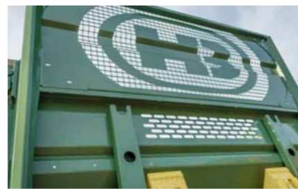
Large protective grid protects against stone chipping and offers optimal visibility into the load compartment
