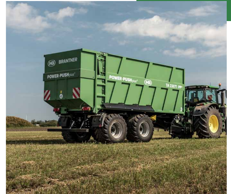
TA 23071 PP+ optionally with hydraulically folding rear underride guard
