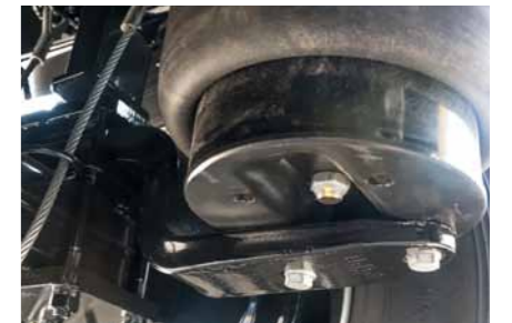
Air suspension with two-leaf link for optimum stability and off-road mobility
