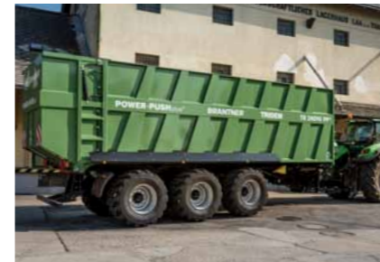
TR 34090 PP+ Tridem chassis, 34 tons total weight, 43 or 49 m 3 load capacity
