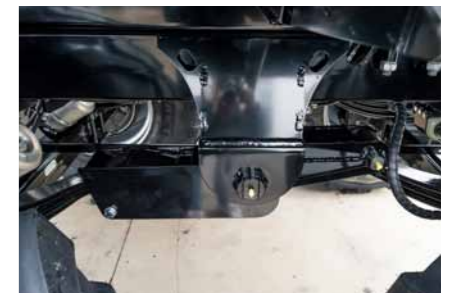
Offset tandem unit suspension adjusted for the steering axle, better stability and reduction of the tendency to roll
