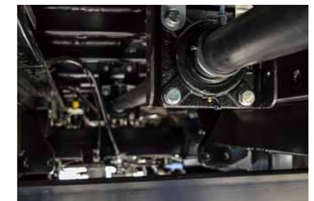
PTO through drive for mounting spreaders or overload snail
