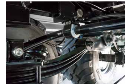
Spring stabilizer highly recommended for steering axles (only possible with parabolic suspension)
