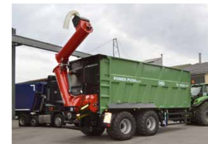
Overload snail hydraulically foldable, with cross auger
