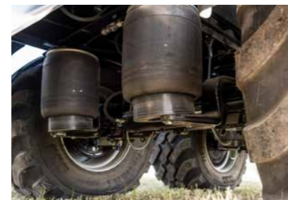
Suspension various systems possible, e.g. air suspension or hydraulic suspension
