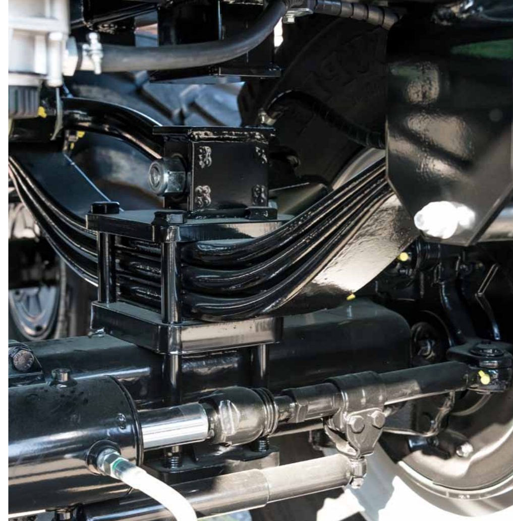
32 to spring unit with reinforced balancing rocker
