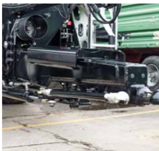
Hydraulic-mechanical forced steering
