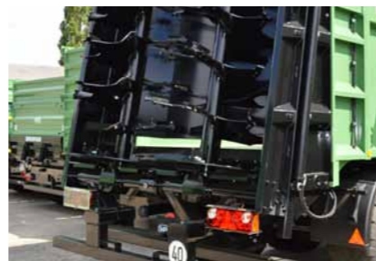
Spread Unit with two vertical high-performance milling drums, screwed-on reinforced milling tines made of Hardox/Quad steel
