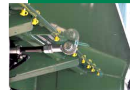
Brantner inovacija Hydraulically controlled pendulum function for opening and closing
