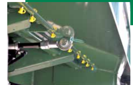
Brantner inovacija Hydraulically controlled pendulum function for opening and closing
